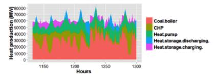
Excessive electricity goes to heat pump Excessive heat goes to heat storage CHP starts to reduce electricity output
