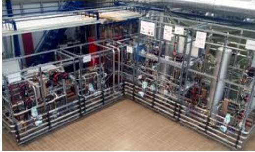
Fig. 1: NODES Lab, a district heating and cooling network at laboratory scale.
